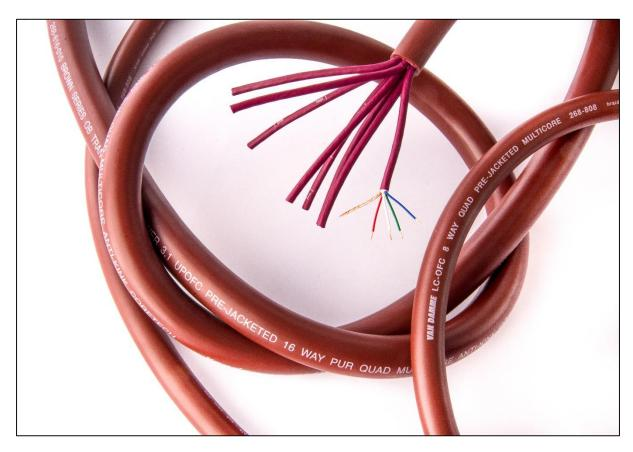
Van Damme Brown Series 8 and 16 pair starquad multicores are the ultimate Outside Broadcast audio cables. Featuring an extremely tough polyurethane (PUR) outer jacket, < 90% coverage individual braided screens for high rejection of EMI and RFI and with overall diameters sized to suit the common outside broadcast multipins. These cables are mechanically and electrically built to excel in the most hostile of environments.
